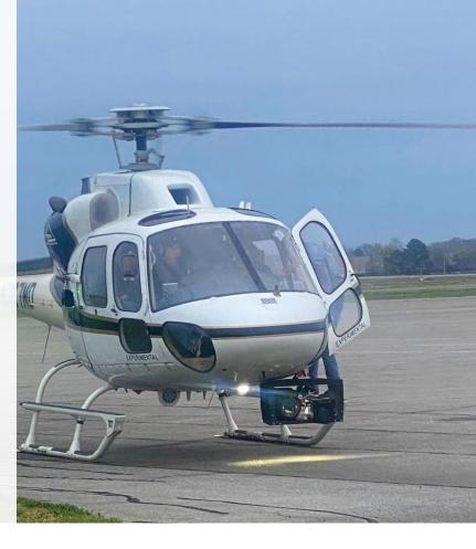
Areté's Lidar for Situational Awareness (LiSA) is a state-of-the-art sensor providing superior pilotage and safety, improving understanding of hazards, wires, obstacles, flight paths and landings in all weather conditions, especially Degraded Visual Environments (DVE). LiSA provides superior range – 2km – and real time 3D spatial awareness of the operational environment and flight guidance at all phases of flight.
